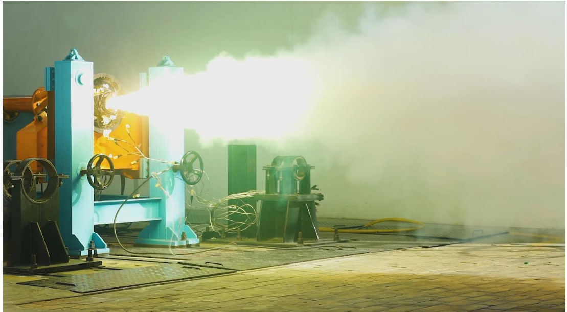
Successful Test fire of the Kalam Motor, qualifying the main three stages of Vikram-1 Launcher
