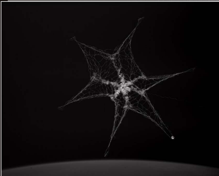
A cube sat targeted and captured by THE NET, then deorbiting together.
